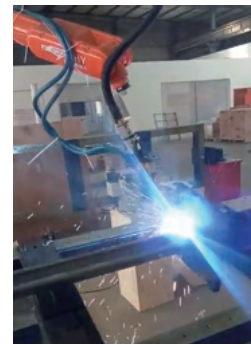
All-around welding of the corner post
