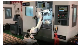
CNC Milling Machine Tending from Front or Side
